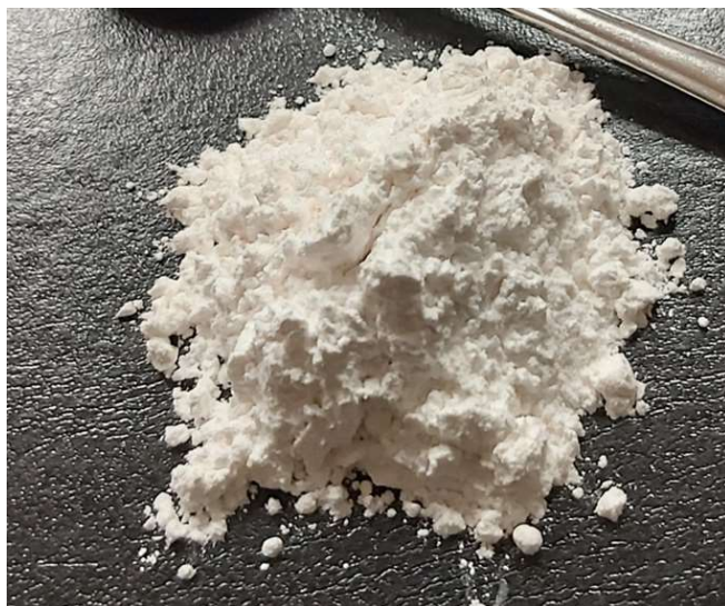
Figure 1. Beharra Leach Residue Calcined Product, 99.94% SiO 2
