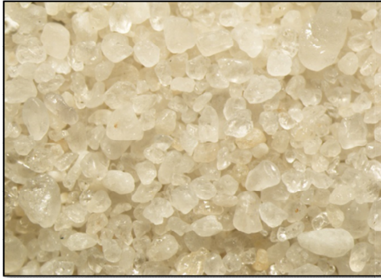
Figure 4. Acid Leach sample 3 with a SiO 2 grade of 99.79.
